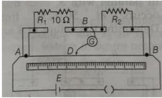
**Q17.** (i) State the principle of working of a meter bridge.
