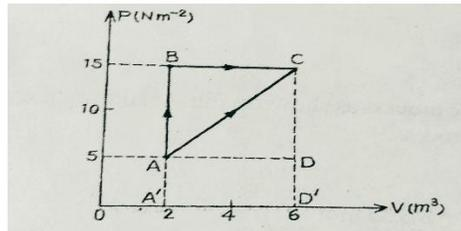
38. In the given figure, an ideal gas changes its state from state A to state C by two paths ABC and AC.
